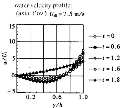
Fig. 4a Axial flow ( $\theta = 70^\circ, \alpha = 0$ )
