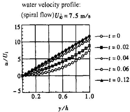
Fig. 8b Spiral flow ( $\theta = 50^\circ$ ,  $\phi = 30^\circ$ )
