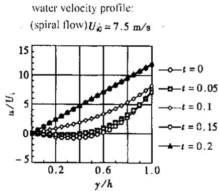
Fig. 4b Spiral flow ( $\theta = 70^\circ, \alpha = 0$ )
