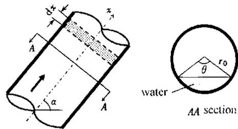
Fig. 2 Geometry of water purging out of an inclined pipe
